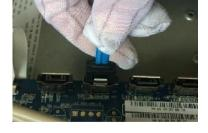
4. Connect the other end of HDD cable to the mainboard.
