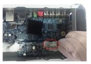
6. (Optional) Pull the battery cable through the hole to connect into the cable port.
