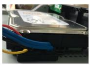
Use the HDD cable and power cable to connect
