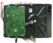
2. Fix the screws on the HDD, but do not be fastened.
