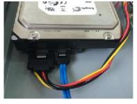
Use the HDD cable and 5. power cable to connect HDD and mainboard.
