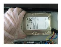
Place the HDD onto the Device.
