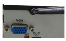
Remove the screws on the rear panel.
