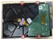
Fix the screws onto the HDD, but do not be fastened.
