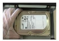
3. Put the HDD into the Device.
