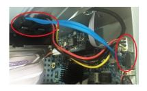
Use the HDD cable and power cable to connect HDD and mainboard.
