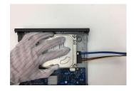
3. Align the screws of the HDD with the holes on the back of the device.
