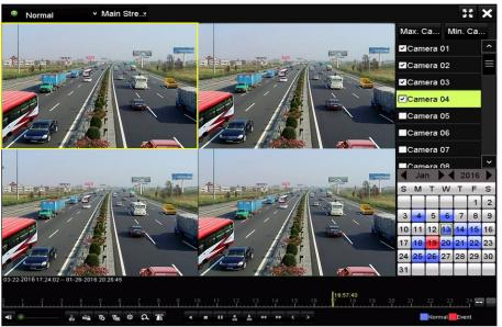
Figure 6-26 4-ch Synchronous Playback Interface
